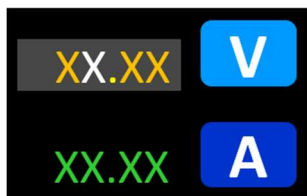
Voltage (V) setting selected and the 'tens' digit being edited.
